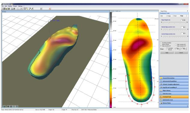
If you want to have it completely flat, select the area required (using the selection tool), adjust "Set Height" from the "Edit" tab, as well as ticking one of the smoothing boxes. Apply.
