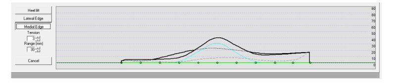
The light Dotted lines represent the internal shape of the orthotic from heel cup to fore foot.
