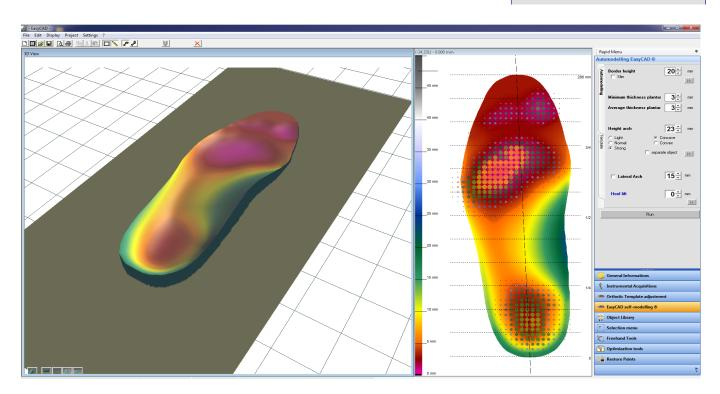
Step 4: Go to Selection Menu click on the Border. This will place a border on your template. You can adjust the height of the border by moving the slider to the left or right. The Medial and lateral junction sliders will decrease or incresse the angle of the junction between the forefoot area and the new Heel border.
