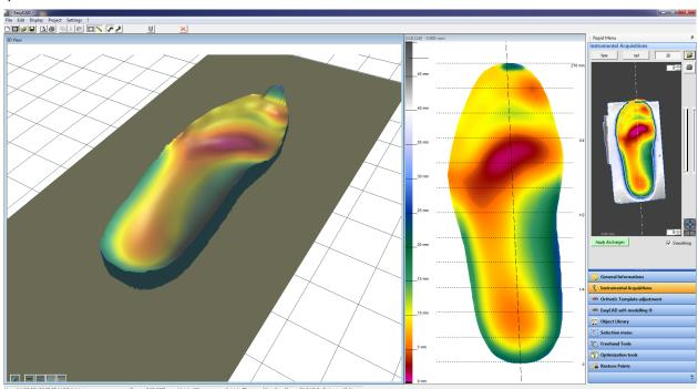
Step 4: Under Selection Menu select the Border on the template and add your border. In general terms, the border does not usually extend beyond the beginning of the arch, but this is at your discretion. Adjust the gradient profile for the border. Select Heel cup contour eq Cubic/Linear etc. Click Apply
